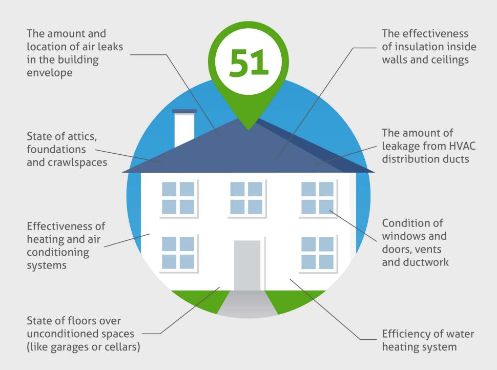
The HERS rating provides a computerized simulation analysis utilizing RESNET Accredited Rating Software to calculate a rating score on the HERS Index. The report will also contain a cost/benefit analysis for the recommended improvements and expected return on investment.
